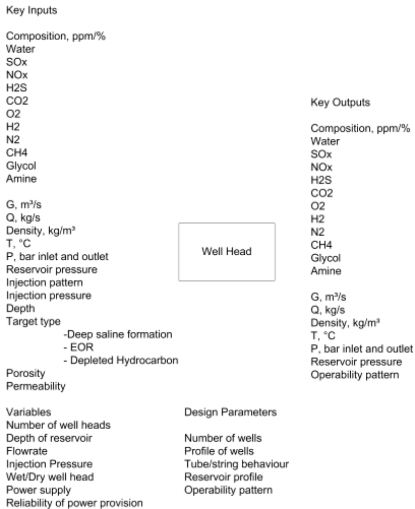
Figure 20 Key inputs, outputs, variables and design parameters for well head component model
