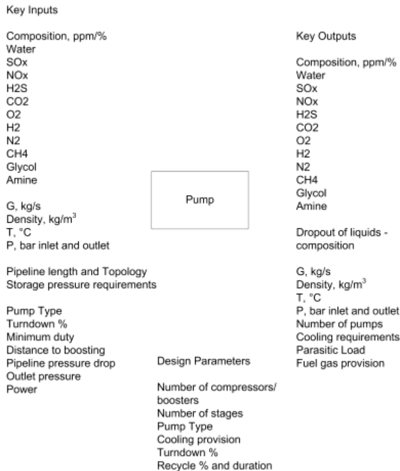
Figure 13 Key inputs, outputs, variables and design parameters for pump component model
