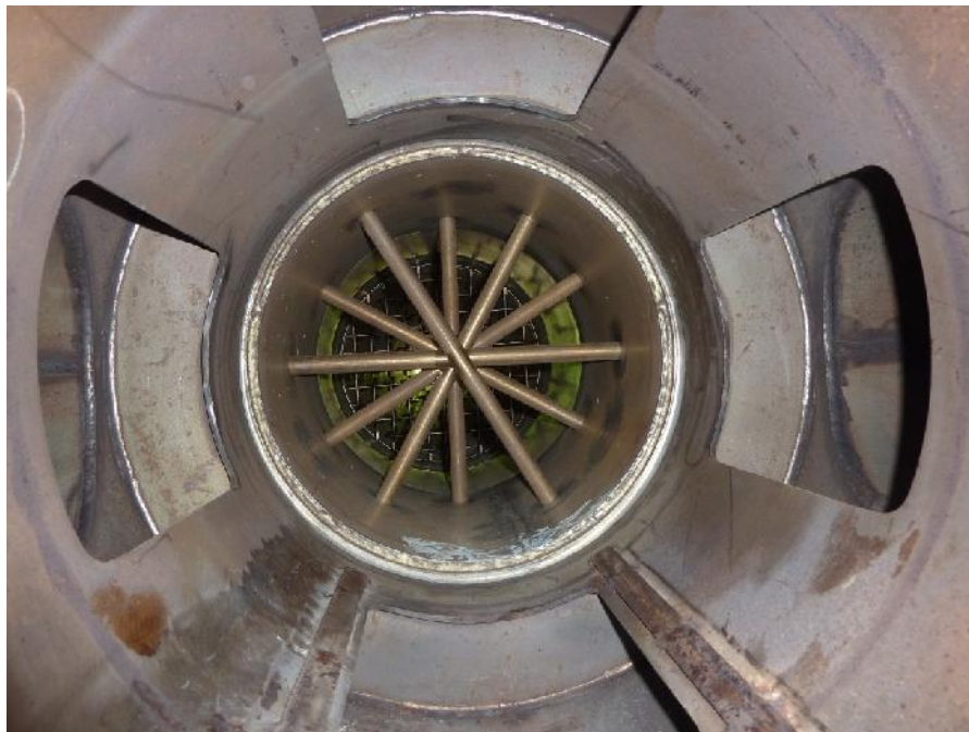
Figure 7: Gas diverter section
