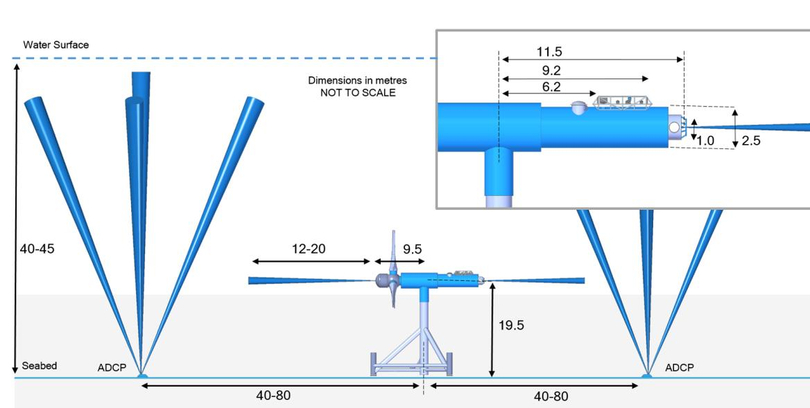
Figure 4: Schematic (not to scale) of the turbine, upstream and downstream ADCPs and ESIP-1 and ESIP-2 mounting positions.
