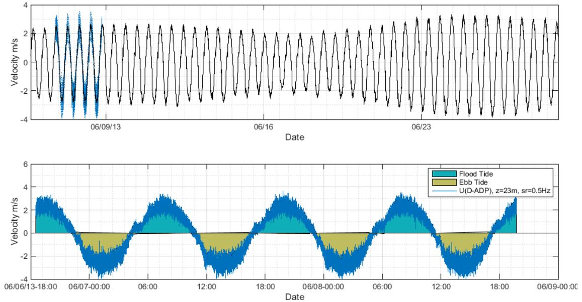
Figure 2: Example of archived data. Tidal cycles (June 2013) from the Fall of Warness, Orkney showing defined Flood and Ebb tidal streamwise velocities. Two data types shown: averaged to 5 minutes (top) and underlying high frequency raw data at 0.5Hz (overlaid and bottom).
