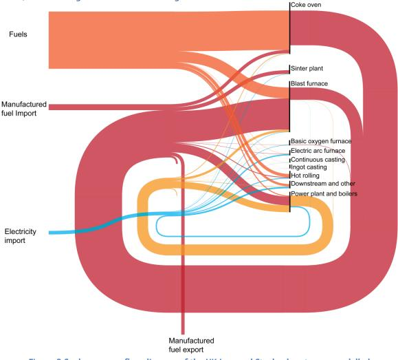
Figure 2 Sankey energy flow diagram of the UK Iron and Steel subsector, as modelled
