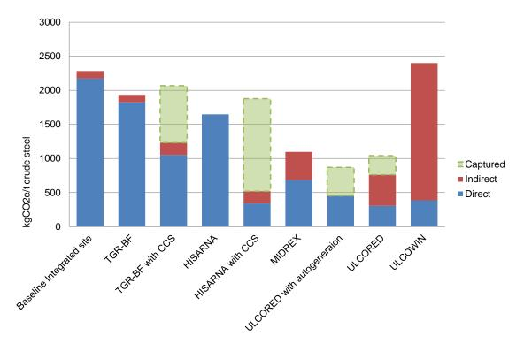
Figure 4 Summary CO<sub>2</sub> emissions intensities of alternative steelmaking systems in the UK (Birat 2012, Birat et al. 2008, IEA GHG 2013a, International Iron and Steel Institute 1998, Link 2008) (Note that TGR-BF, HISARNA and ULCORED consume significantly more oxygen than the base case which would show slightly high indirect emissions if incorporated).
