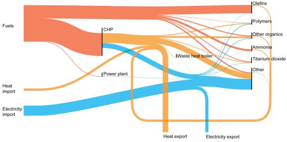
Figure 6 Sankey energy flow diagram of the UK Chemicals subsector as modelled.
