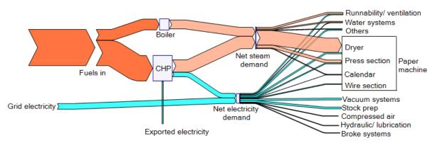
Figure 8: Sankey diagram of Paper subsector.
