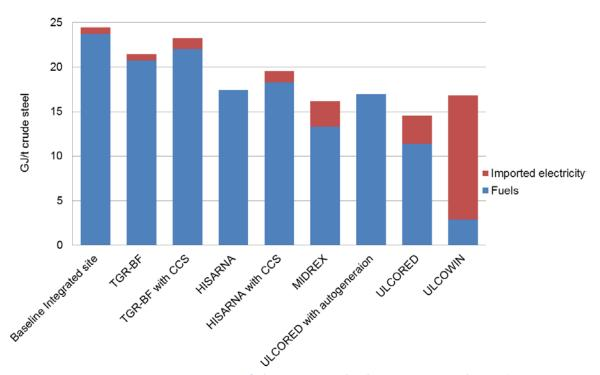
Figure 3 Summary energy intensities of alternative steelmaking systems in the UK (Birat 2012, Birat et al. 2008, IEA GHG 2013a, International Iron and Steel Institute 1998, Link 2008). (Note that TGR-BF, HISARNA and ULCORED consume significantly more oxygen than the base case which would show slightly higher imported electricity if incorporated).
