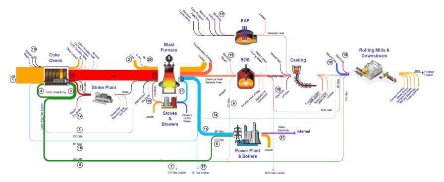
Figure 1: Simplified Sankey diagram of the UK iron and steel subsector (DECC 2011) (This diagram was not produced from the analysis in this project and is based on the year 2009.)
