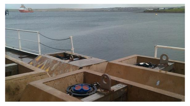
Figure 3: Multiple ADCP D-ADP's quayside in Orkney, UK prior to deployment in 2014
