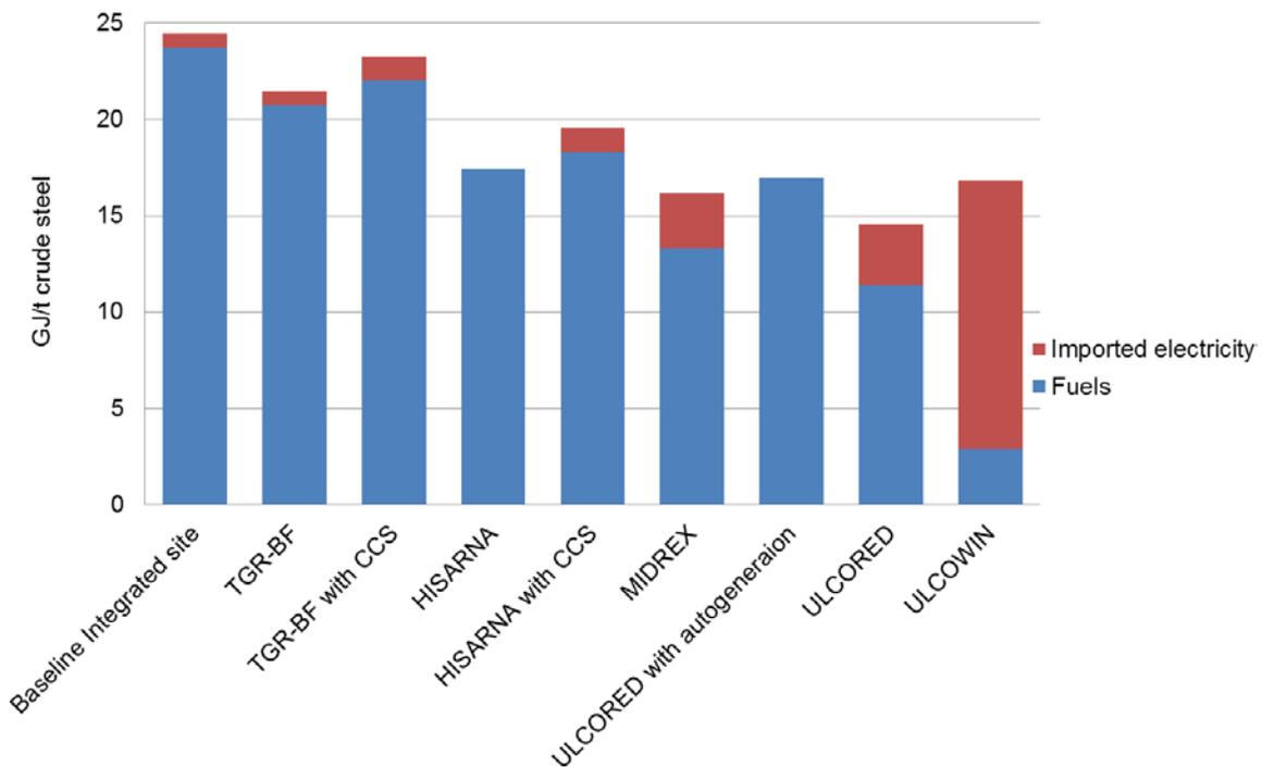
Figure 3 Summary energy intensities of alternative steelmaking systems in the UK (Birat 2012, Birat et al. 2008, IEA GHG 2013a, International Iron and Steel Institute 1998, Link 2008). (Note that TGR-BF, HISARNA and ULCORED consume significantly more oxygen than the base case which would show slightly higher imported electricity if incorporated).
