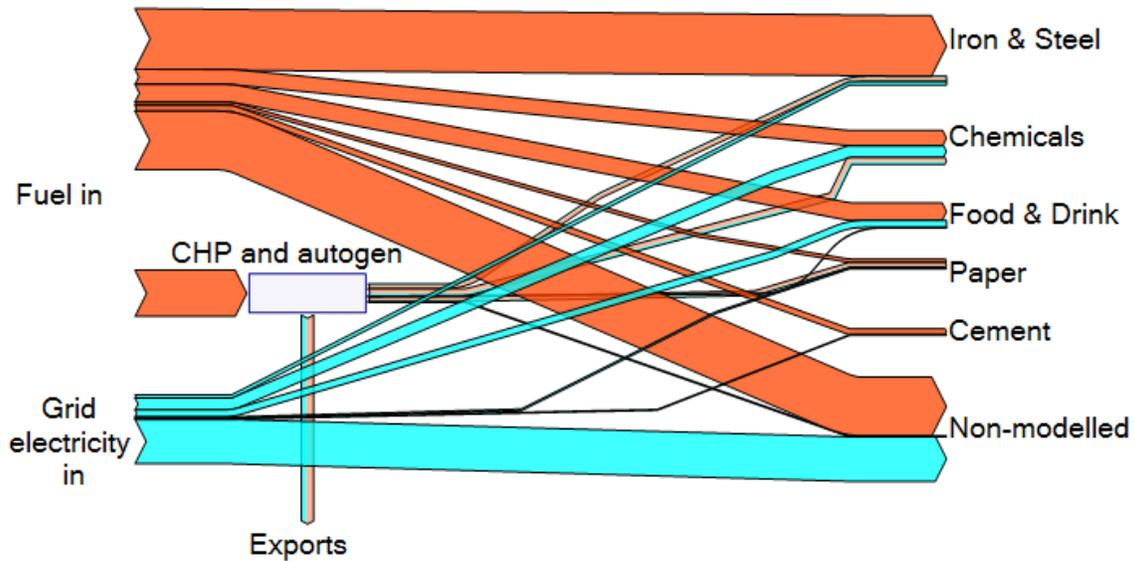
Figure 10: Sankey diagram of modelled and non-modelled subsectors of industry.
