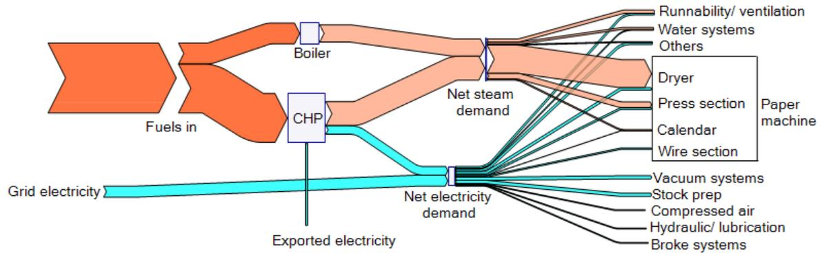
Figure 8: Sankey diagram of Paper subsector.
