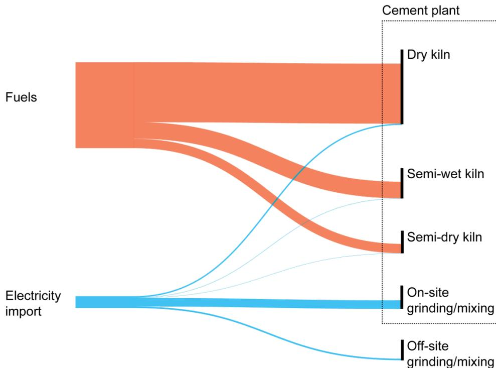
Figure 9 Sankey energy flow diagram for the UK Cement subsector as modelled (CSI 2013, MPA 2011).
