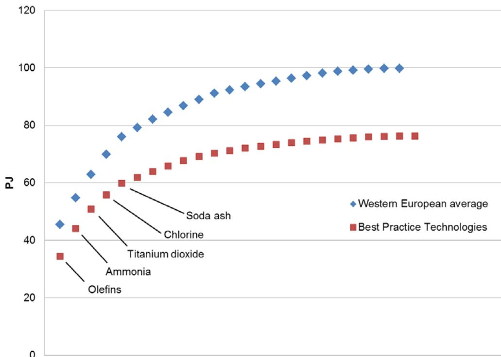
Figure 5 Final energy demand (Fuel, electricity and steam) from modelled processes applying average Western European and best practice technology efficiencies to estimated UK production (APPE 2013, DECC 2013a, ICIS 2013, IEA 2009b).
