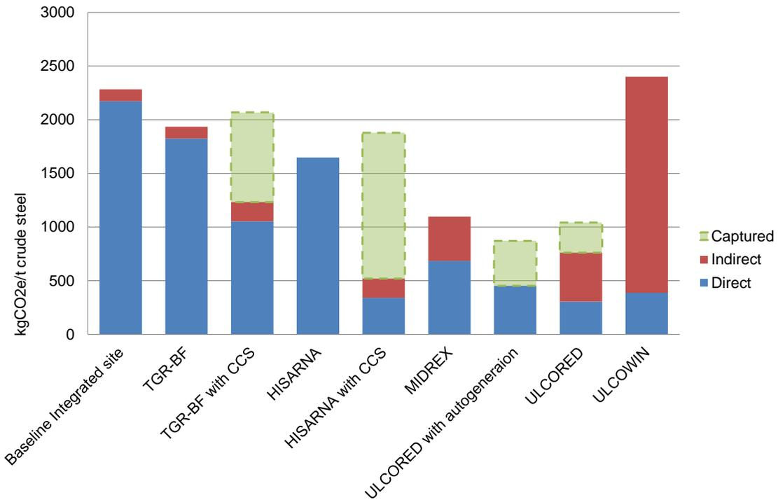
Figure 4 Summary CO<sub>2</sub> emissions intensities of alternative steelmaking systems in the UK (Birat 2012, Birat et al. 2008, IEA GHG 2013a, International Iron and Steel Institute 1998, Link 2008) (Note that TGR-BF, HISARNA and ULCORED consume significantly more oxygen than the base case which would show slightly high indirect emissions if incorporated).
